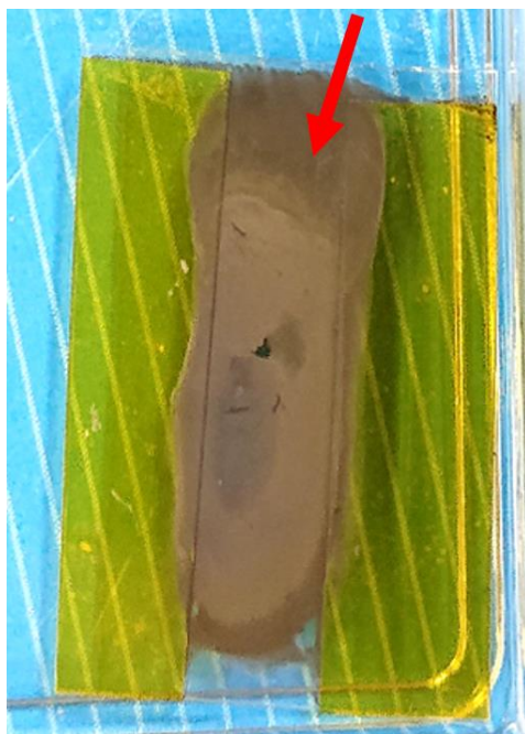
Figure 3-21. Optical image of the brown Cu/Ag thin film obtained by dipping Cu@Ag NPs into the 29 mM HCl methanol solution for 30 min at RT.
